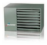
Modine's PTS/BTS separated combustion unit is specifically designed for greenhouse environments and their hostile atmospheric conditions, such as chemicals, high humidity and negative pressure. This tubular heat exchanger is available in units rated from 150,000 to 400,000 BTU/hr. On these units, combustion air is brought in from outside the heated area, either from outdoor air or from an adjacent room, eliminating the need to use contaminated indoor air for combustion.
